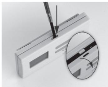
compartment. After the batteries have been inserted, the display flashes the measured room temperature. (If this information fails to appear on the display, press the „**RESET**” button located on the main panel of the thermostat.
